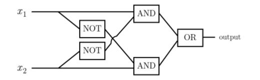
Any Boolean function  $f : \{0, 1\}^n \rightarrow \{0, 1\}^m$  is computable by a Boolean circuit C using just AND, OR, and NOT gates. i.e., AND, OR, and NOT gates are universal.
