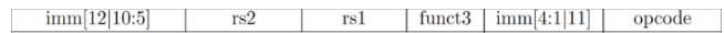
Figure 7: B-type instruction structure for RISC-V, rs1 and rs2 are the source registers for branch operation.
