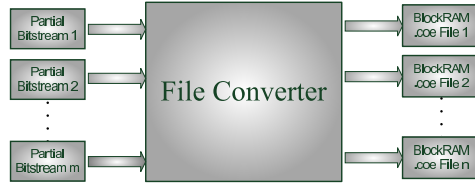
Fig. 5. File conversion from partial bitstream file to BlockRAM coefficient file
